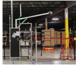
(c) KIVA Systems' inventory station and drive robot
