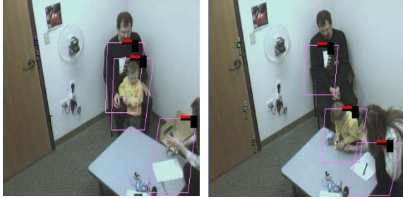
Figure 2: Using a calibrated pair of stereo cameras, we can successfully locate and track individuals as they move throughout one of our clinical evaluation rooms during an interview session. Pairs of stereo images are used to compute a disparity image which is combined with information on color, direction of motion, and background models to identify and track individuals moving throughout a room.
