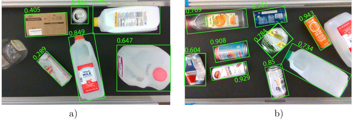
Figure A.8: Sample Qualitative Results from our Robot System: Similarity scores of objects on the conveyor belt obtained from our method, when the human trained the system with 30 objects of type a) half-gallon milk jugs b) un-crushed cans
