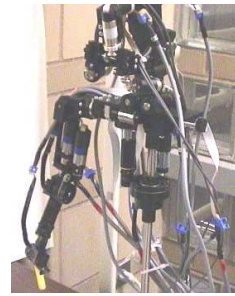
Figure 1: Nico, the physical robot that performed the self-recognition task.
