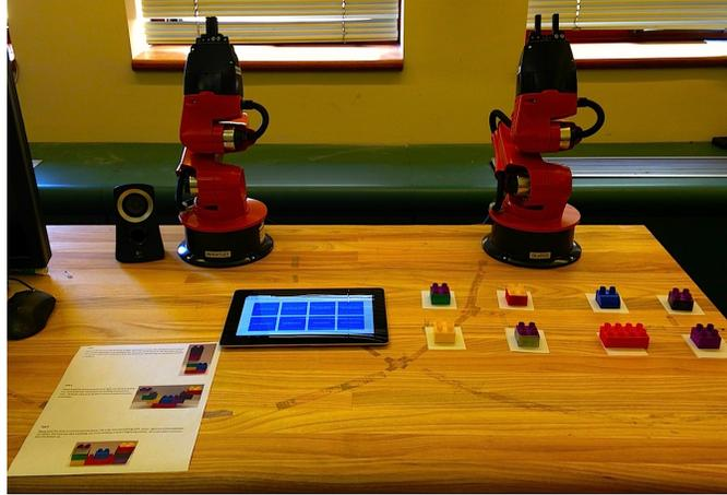
Figure 2.7: Collaborative Workbench platform with experimental setup, used to learn task structure from demonstrations of construction activities.
