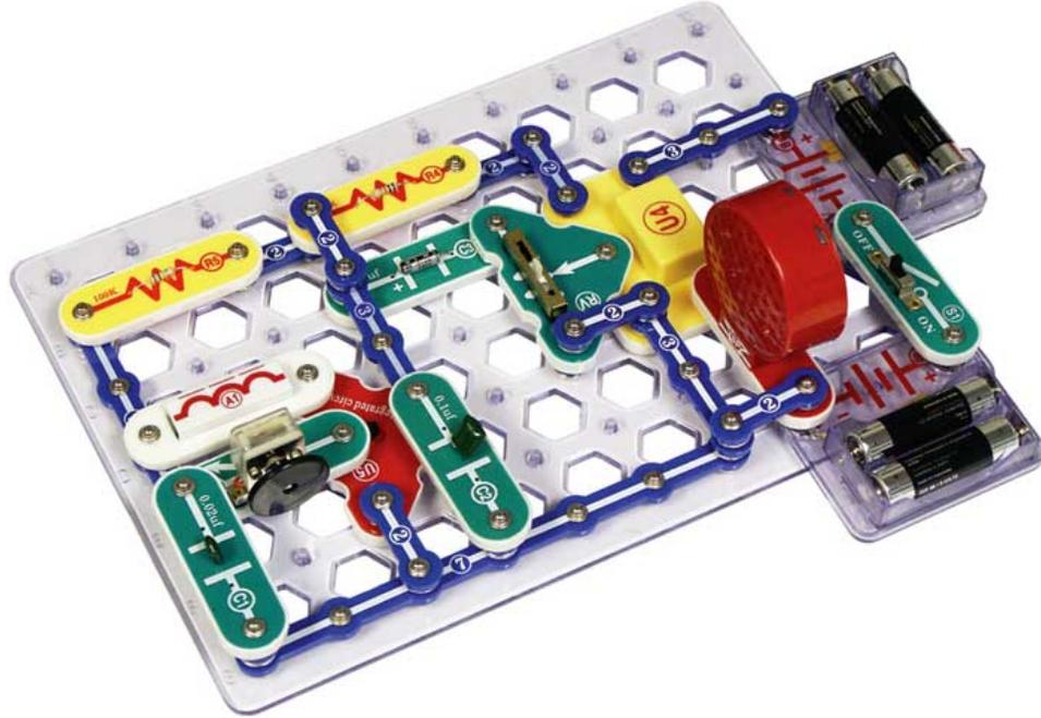
Figure 3.4: Example of a SnapCircuits solution. Snap buttons indicate valid connection points between components, which must be joined to form circuits in a manner that satisfies the implicit 3D spatial constraints imposed by the pieces available and the desired goal circuit function.
