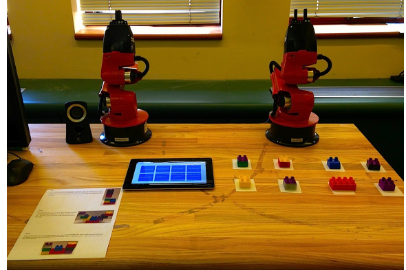
Fig. 1. Collaborative Workbench platform with experimental setup, used to learn task structure from demonstrations of construction activities.
