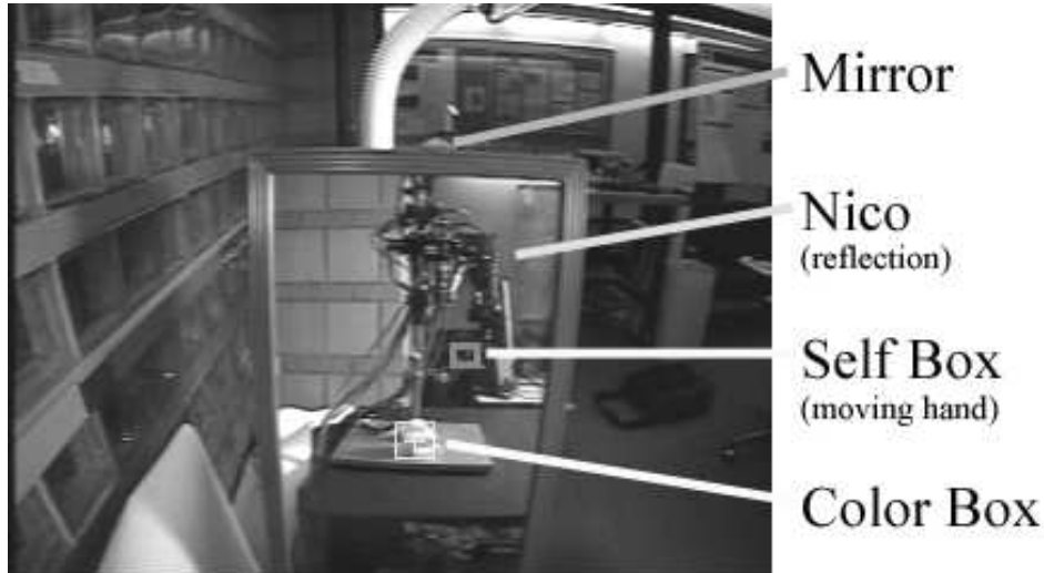
Figure 5.9: A view of the setup of Gold and Scassellati (2006c), taken from one of Nico’s cameras. The robot can see its reflection in the mirror, center. Superimposed on the image is the bounding box produced by the “color” module, which has found the mirror reflection of the bright yellow ball, and the box produced by the “self-motion” module, which has found the reflected motion caused by Nico’s arm movement.
