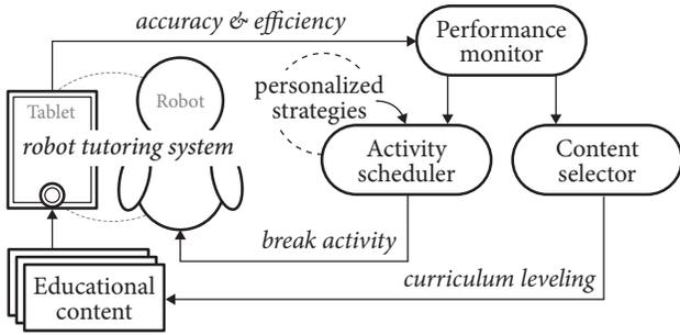
Figure 2: System architecture of our robot tutoring system.
