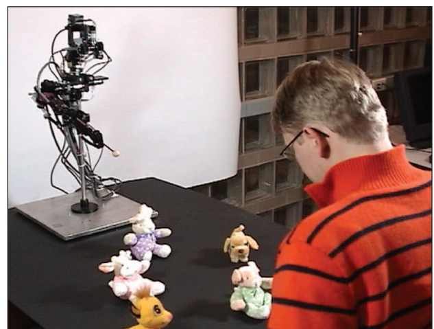
FIGURE 1 A humanoid robot (named Nico) uses a learned pointing behavior to acquire joint attention skills. When the robot points to one of the objects lying in front of it, the caregiver will very likely look at what the robot is pointing to. The robot learns to associate spatial positions with head postures and can then extrapolate from a head posture to a location in the world.
