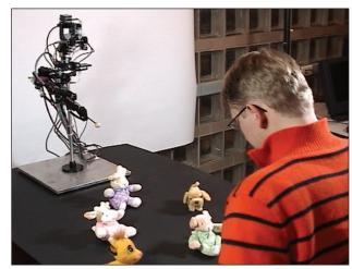
FIGURE 1 A humanoid robot (named Nico) uses a learned pointing behavior to acquire joint attention skills. When the robot points to one of the objects lying in front of it, the caregiver will very likely look at what the robot is pointing to. The robot learns to associate spatial positions with head postures and can then extrapolate from a head posture to a location in the world.
