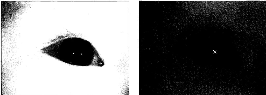
Figure 2.2: Rule-based Pupil/Corneal Reflection Detection. *Left*: image from the eye camera (Singer-Vine, 2008). *Right*: simple rule-based heuristics localizing the pupil (red), pupil-center (yellow x), and centers of corneal reflections (cyan cross).
