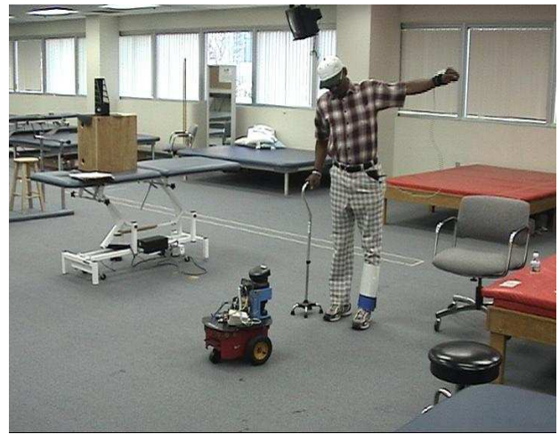
Fig. 2. Therapist robot encouraging and monitoring stroke patient during the rehabilitation therapy (work done at USC [12])
