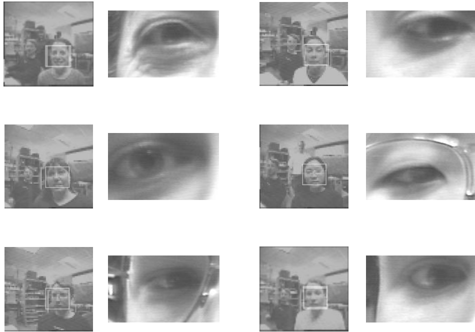
Figure 4: Examples of successful face and eye detections. The system locates faces in the peripheral camera, saccades to that position, and then extracts the eye image from the foveal camera. The position of the eye is inexact, in part because the human subjects are not motionless.
