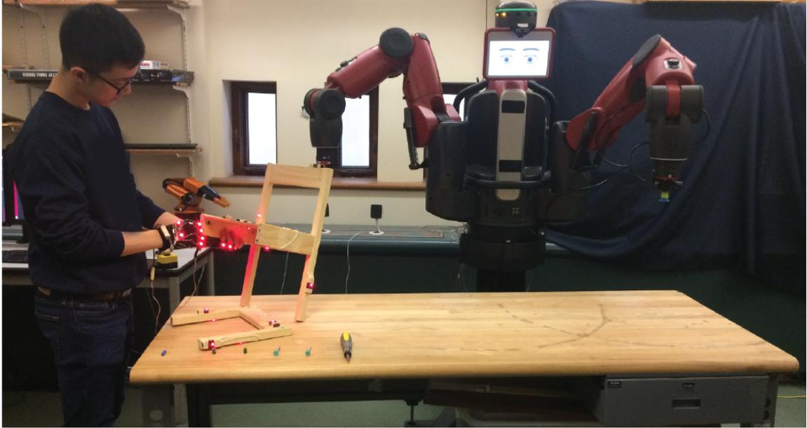
Figure 3.1: Participant assembling an IKEA chair during data collection. We use a motion capture system to record the participant’s hand movements (via gloves fitted with sensors), and the trajectories of the chair components.
