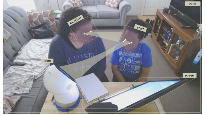
Fig. 4: Target Detection. Attentional targets are estimated by the intersection of one’s visual cone and static object locations.
