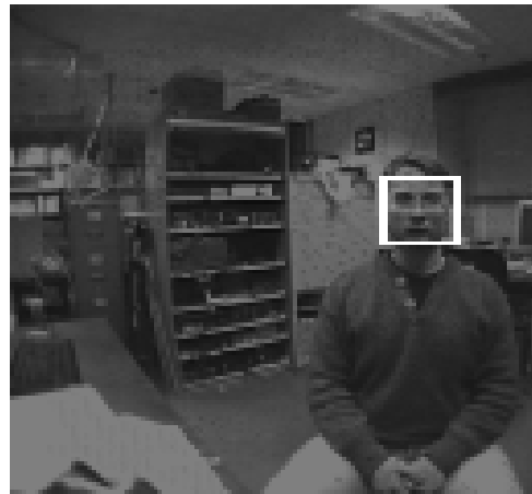
Figure 3: An example of the face detector. The 128x128 grayscale image was captured by the active vision system, and then processed by the pre-filtering and ratio template detection routines. One face was found within the image, and is shown outlined.
