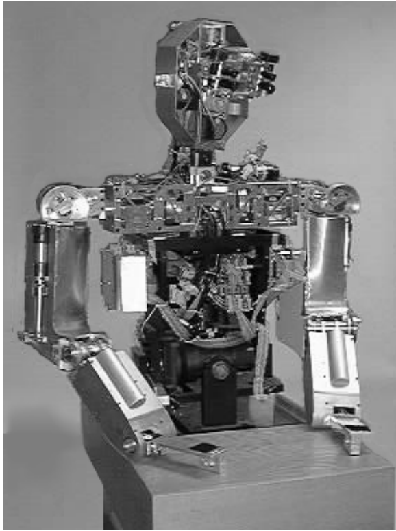
Figure 1: Cog, an upper-torso humanoid robot. Cog has 21 degrees of freedom to approximate human motion, and visual, vestibular, proprioceptive, and auditory senses to approximate human perception.
