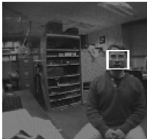
Figure 3: An example of the face detector. The 128 \times 128 grayscale image was captured by the active vision system, and then processed by the pre-filtering and ratio template detection routines. One face was found within the image, and is shown outlined.
