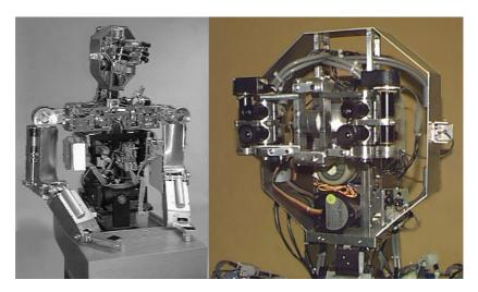
Fig. 1. Cog, an upper-torso humanoid robot. Cog has twenty-one degrees of freedom to approximate human movement, and a variety of sensory systems that approximate human senses, including visual, vestibular, auditory, and tactile senses.
