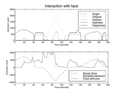
**Fig. 9.** Experimental results for Kismet interacting with a person's face. When the face is present and moving slowly, the robot looks interested and happy. When the face begins to move too quickly, the robot begins to show disgust, which eventually leads to anger.
