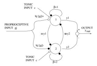
Fig. 6. Schematic of the oscillator. Black circles correspond to inhibitory connections, open circles to excitatory. The  $\beta v_i$  connections correspond to self-inhibition, and the  $\omega y_i$  connections give the mutual inhibition. The positive and negative parts of the input  $g_i$  are weighted by the gain  $h_i$  before being applied to the neurons. The two outputs  $y_i$  are combined to give the oscillator output  $y_{out}$ .
