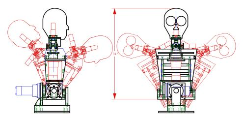
Fig. 2. Range of motion for the neck and torso. Not shown are the neck twist (180 degrees) and body twist (120 degrees)
