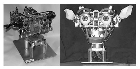
**Fig. 3.** Two of the vision development platforms used in this work. These desktop systems match the design of the Cog head and are used as development platforms for visual-motor routines. The system on the right has been modified to investigate how expressive facial gestures can regulate social learning.
